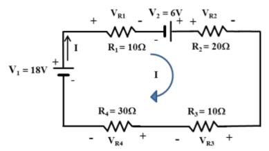
Apply the Ohm's law to define the voltages, or voltage drops, across the four resistors. **Note:** since all four of the resistors are in series, we *could* combine them into a single REQ before applying KVL. However, in this case we will keep resistors separate just to maintain consistency with the approach adopted in Example 2.2.
