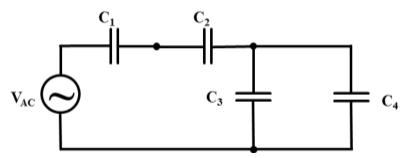
As computed in problem 6, the combined or net capacitance contributed to the circuit by the parallel and series network of capacitors is  $C_{EQ} = 4.44 \mu$ F. Then, by applying Eq.1.26:
