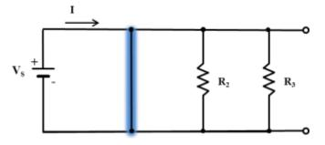
The highlighted segment in the circuit above represents the short circuit that replaces  $\mathbf{R}_1$ . Since  $\mathbf{R}_1$  is replaced by a short circuit - regardless of the disposition of other circuit elements - it becomes a *path of least resistance* for the entire circuit. In other words, the voltage source is short-circuited. Interpreted in terms of the Ohm's law, this would mean:
