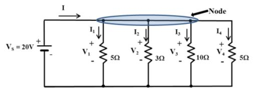
Subscribing to the definition of a node as a point where three or more conductors merge, the shaded segment in the diagram above is designated as the node for this circuit. Then, before applying KCL to determine the source current - using the Ohm's law – define the individual currents through each of the resistors, in terms of the specific resistance values and the voltages around them:
