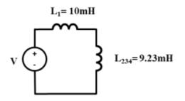
Inductors  $L_1$  and  $L_{234}$ , in this reduced circuit, lend themselves to a linear combination. Therefore, the equivalent inductance  $L_{EQ}$  for the entire parallel and series inductor hybrid circuit would be:
