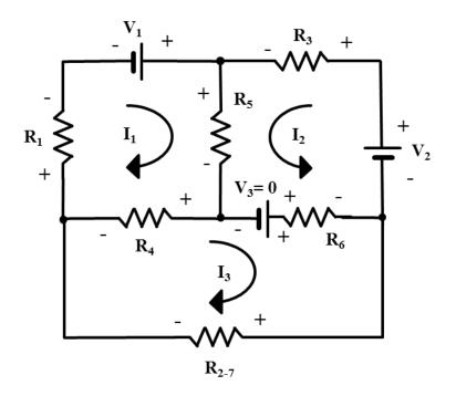
The three simultaneous equations derived by applying KVL to loops 1, 2 and 3, as described in Example 2.5, are:
